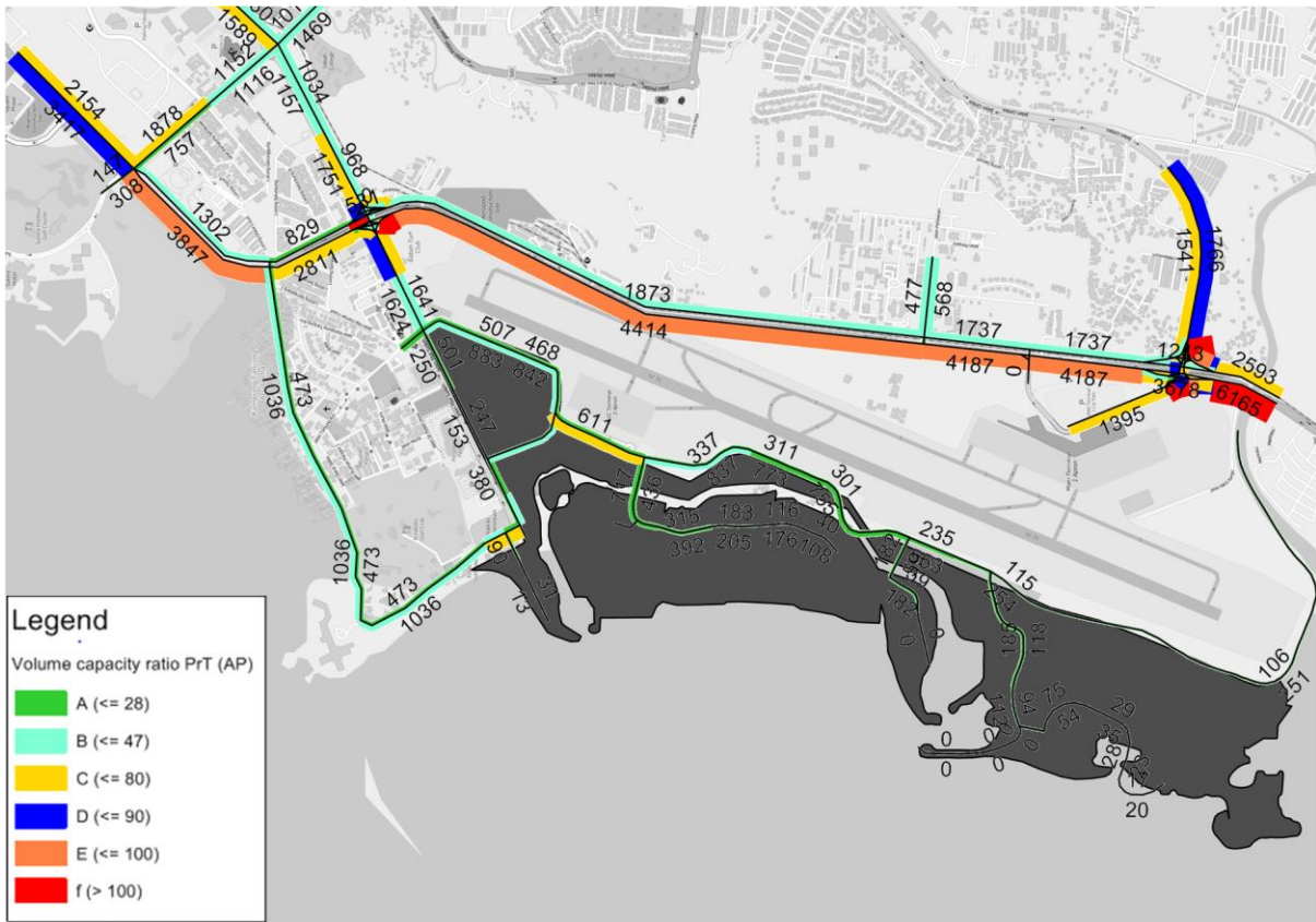
FIGURE 6-4 YEAR 2025 V/C RATIO AT WEEKDAY AM PEAK HOUR WITH TAED AND WITH PUBLIC TRANSPORT
