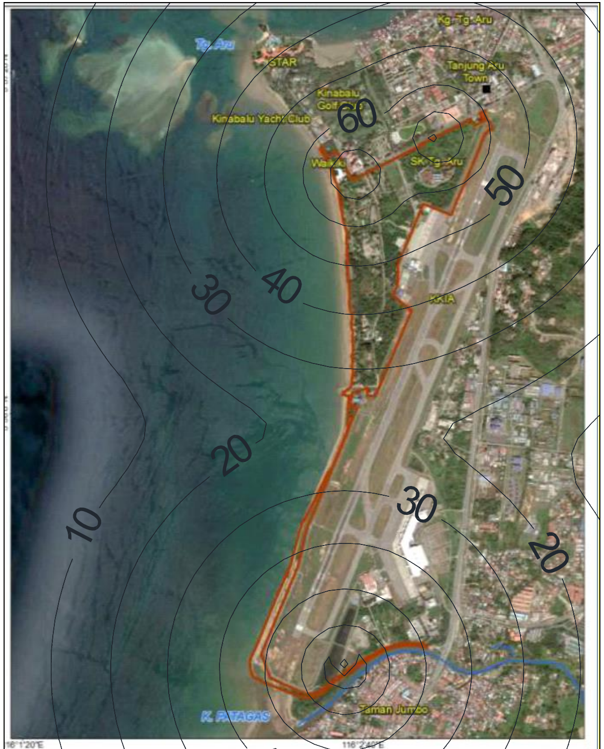
Figure 1: Predicted Noise Source Emission Contours (10 dBA interval) during Sub-Phase 1: Demolition & Site Clearing
