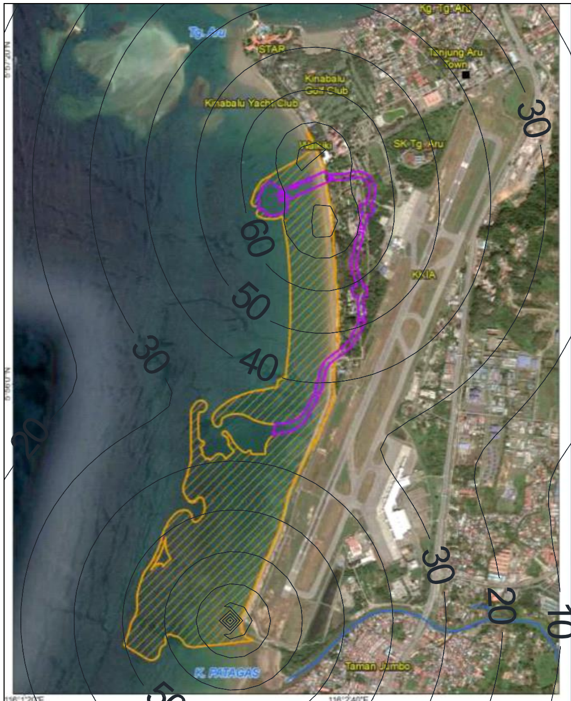
Figure 2: Predicted Noise Source Emission Contours (10 dBA interval) during Sub-Phase 2: Reclamation & Dredging
