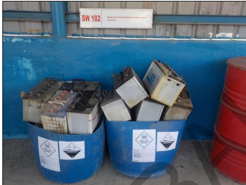
Plate 14.2: Storage of scheduled waste (SW 102).
