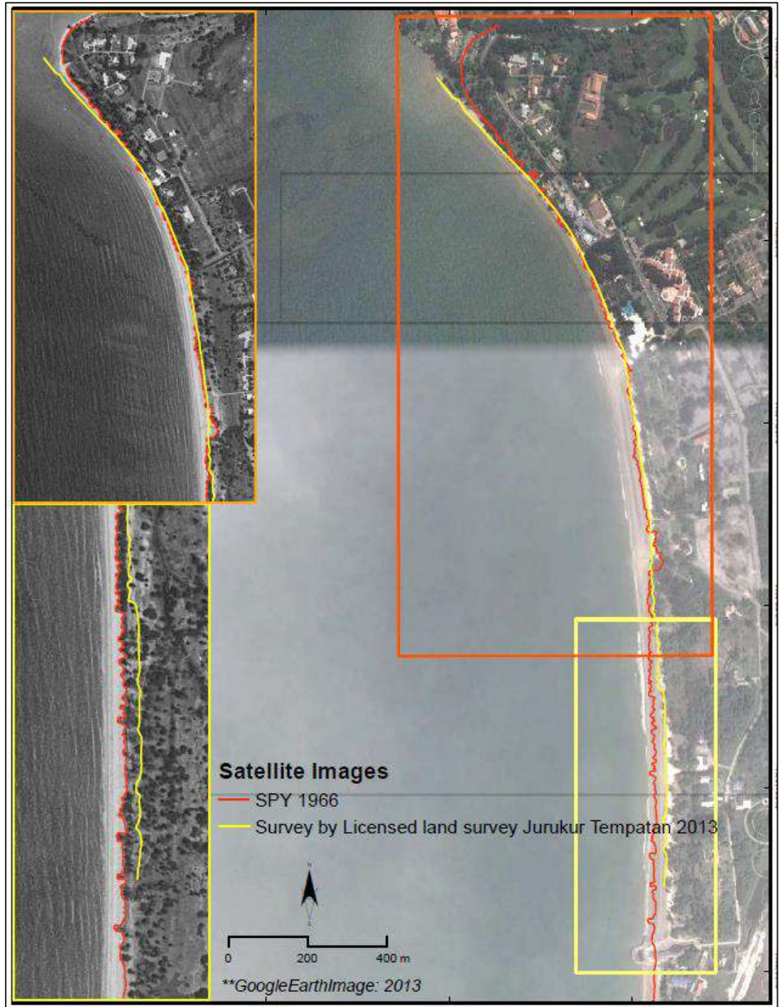
Figure 3.2 1 st , 2 nd and 3 rd beach shoreline erosion over the period of 48 years.
